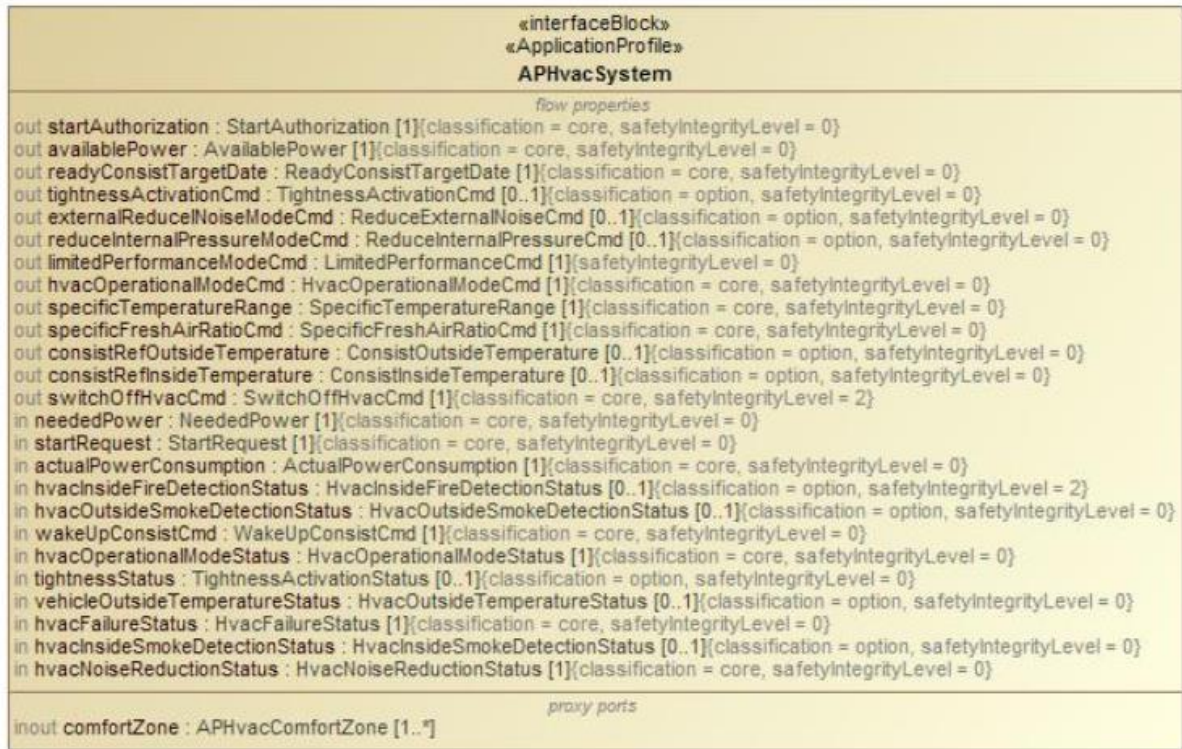
Figure 6: APHvacSystem, one of the Interface Blocks of the Functional HVAC AP (Example from [2])
